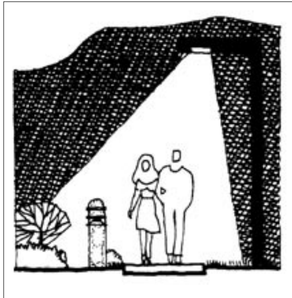
figure 7.2: Pedestrian Area Utilizing Overhead and Bollard Lights
